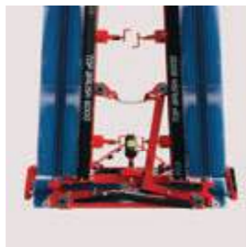
Wings float and pivot to handle undulations.
