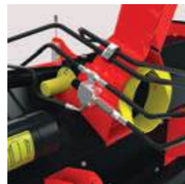
Adjustable conveyor speed to control the rate of material flow.
