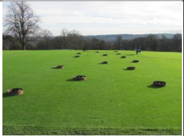
Plate 10: Water infiltration measurement
