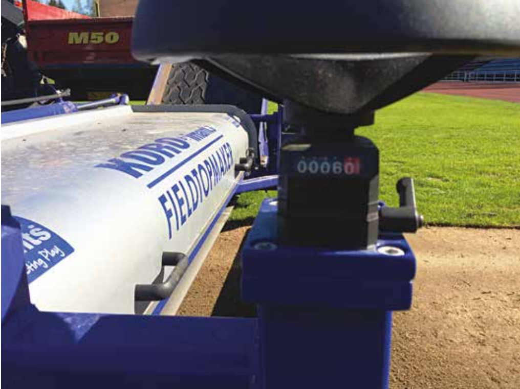
Depth setting is accurate to 0.5mm, via a digital display read out
